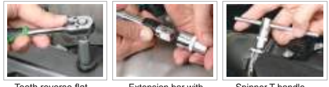
Teeth reverse flat ratchet handle Extension bar with quick release Spinner T handle
