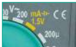
1.5V Battery Test
