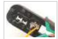
Strips twisted pair wire
