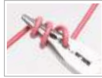
Pulling/Rolling Ø1.6mm/2.0mm copper
