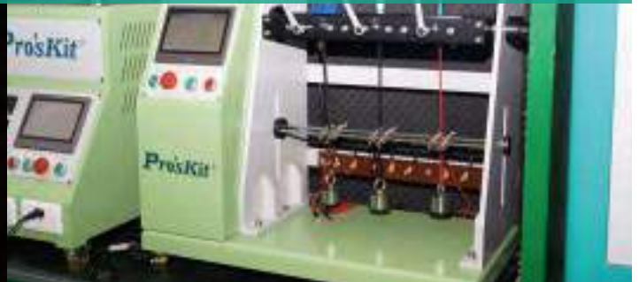
Dial / Knob Switch Fatigue Test
