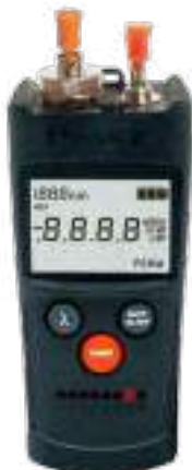
Fiber optic power test
