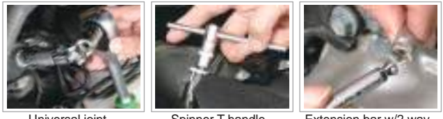
Universal joint Spinner T handle Extension bar w/2 way
