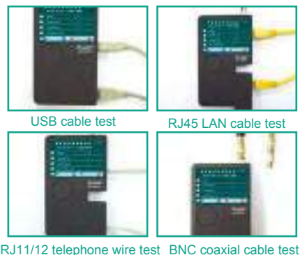
USB cable test RJ45 LAN cable test RJ11/12 telephone wire test BNC coaxial cable test
