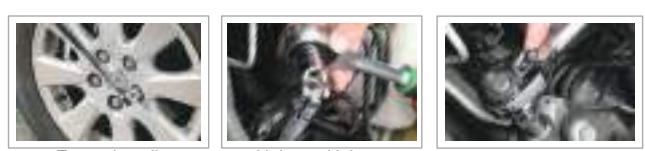
F type handle Universal joint Teeth reverse flat ratchet handle
