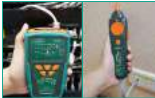
Verify LAN/ telephone cable condition
